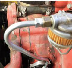
Install the provided fuel line between the fuel pump and the fuel filter. Do not allow the brass fitting on the fuel pump to turn.
