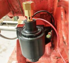
Start the installation by removing the original fuel pump. Save the 90° fitting and the flexible fuel line to reuse with your new electric pump.
